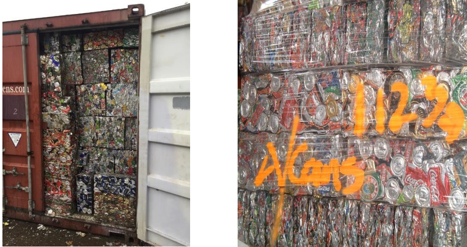
Figure 1: Photos showing aluminium cans ready for export -note the quality of bale at <1% contamination
